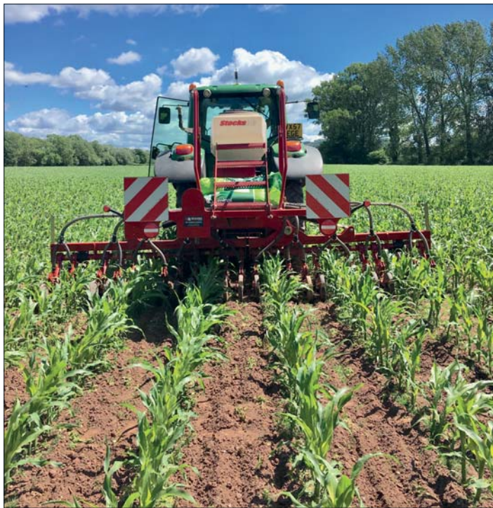
The custom-built drill designed specifically for undersowing maize
